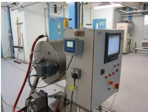
Crucially for process development and pilot work, a data recorder charts a range of Biomixer parameters including power consumption, pH, temperature and shaft rotation speed. This inline monitoring provides invaluable information for process optimisation in relation to substrate characteristics over time and overall energy efficiency. Moreover, the plug and play nature of the Biomixer design allows for new probes to be installed and their outputs recorded with a minimum of down time.
